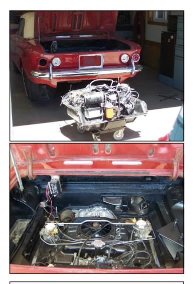
Here's a couple of pictures of Art's 64 engine going back in. After a 2nd trip up to his garage with all the needed bolts and parts it went in like a dream. We had to pull the starter off and clean all the connections and then she fired right off. Now for some exhaust and a front perimeter seal and she'll be ready to go. He needs some brake work and a few other things done before she hits the road. It's coming along good. Ron Thompson
