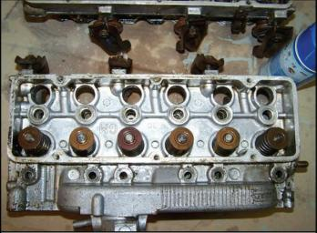
I bought a blue can off Easy Off Oven cleaner and sprayed it on this head. First I knocked all the big stuff off then a quick bath in the parts washer. Next I sprayed it down with Easy Off and let it sit for about 15-20 mins. I hosed it off and here is the results with almost no brushing or cleaning at all. The heads shine like new. Next is a little digging at the dirt that's left the spray again and blast it with the pressure washer. Make surer you wear rubber gloves and eye protection.
