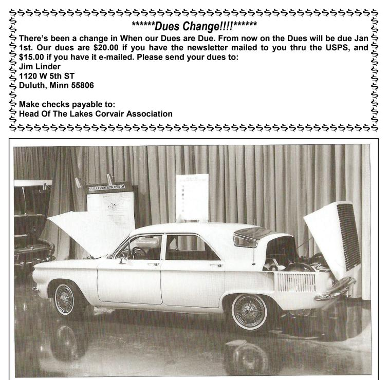
Not all adaptations of the Corvair were sporty. GM used the Corvair as a basis for its "Calvair," a vehicle powered by a Stirling engine which drew heat from a stored supply—thus the "Cal" for "calories." Bizarrely the GM Research engineers equipped this unique fastback Corvair with optional wire-wheel trim covers.
